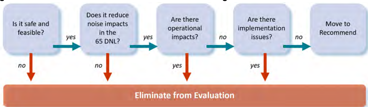
Figure 1 Noise Abatement Alternative Screening Process
